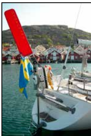
Najad 373 Off-center installation
